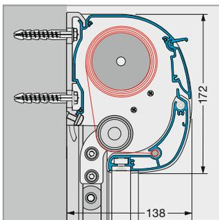
The MICRO 300 is supplied as standard with motor drive.
